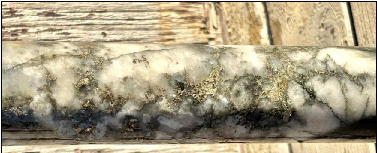
FIGURE 10.8 SULPHIDE MINERALIZATION OF BRECCIATED QUARTZ VEIN IN DRILL HOLE 25UND002
