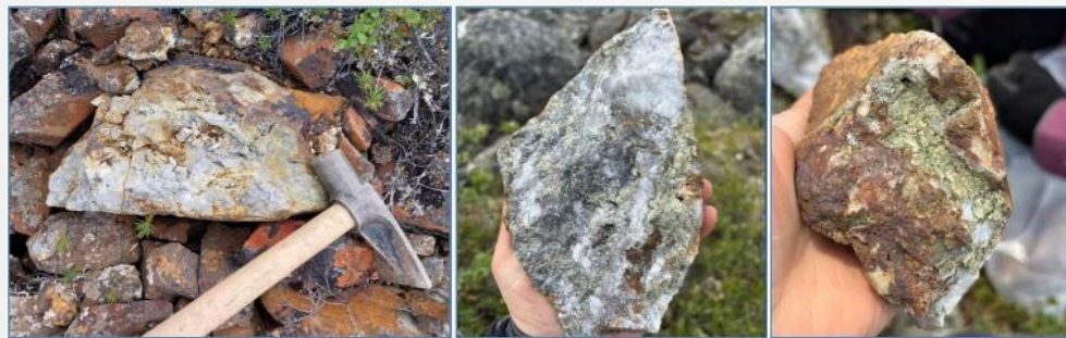
Rock samples from Penny Lane prospect showing chalcopyrite rich quartz veining.
